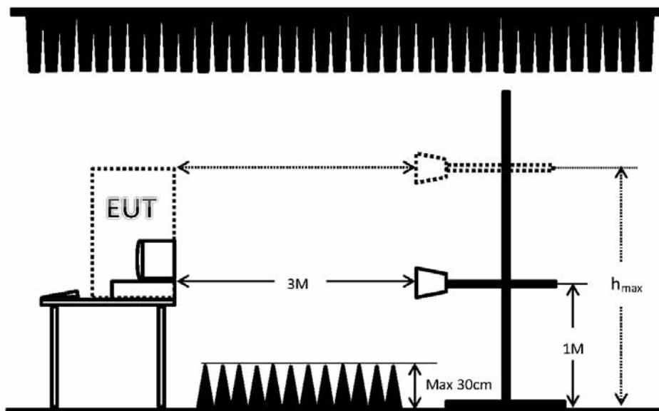
Remark: When EUT's height is over 172cm, h<sub>max</sub> = top of EUT
