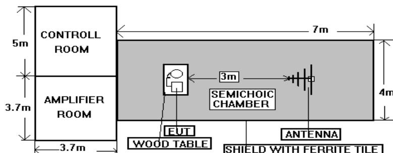
**NOTE :** The SPORTON 7m x 4m x 4m semi-anechoic chamber is compliance with the sixteen point's uniform field requirement as stated in IEC 61000-4-3 Section 6.2.
